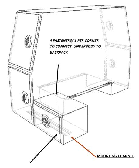
8 FASTENERS FROM MOUNTING CHANNEL TO UNDERBODY & BACKPACK
