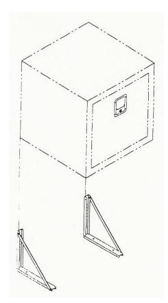
In order to properly support your underbody toolbox, we recommend the use of bottom support mounting brackets.
